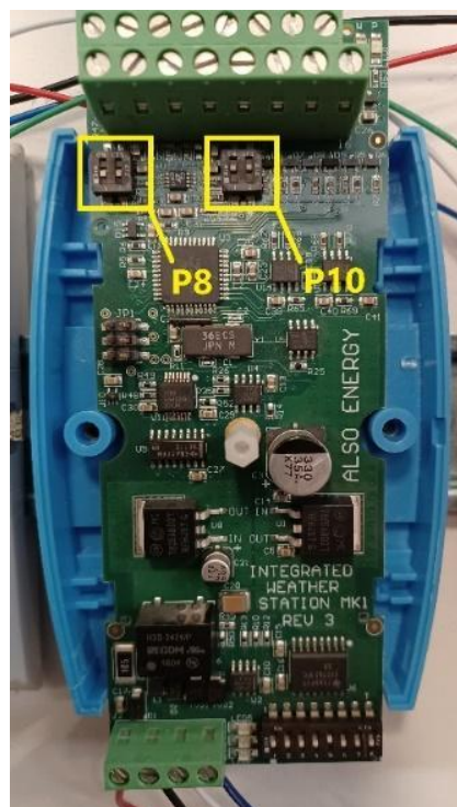
Figure 43: IWS Board Highlighting Gain Switches
