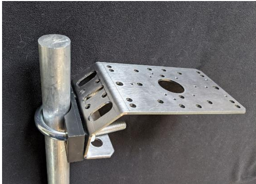
Fig 31 Mounted tangential to pole
