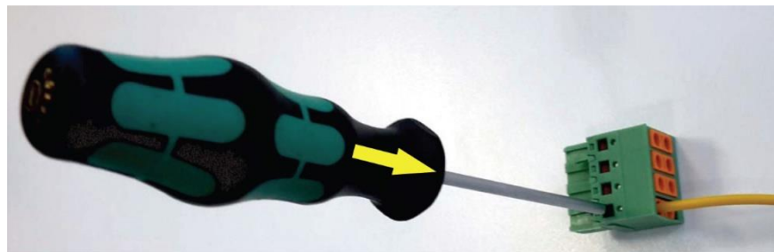
Fig 16 Preparing connectors X4 and X5
