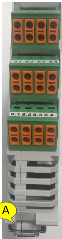
Fig 16 Preparing connectors X4 and X5
