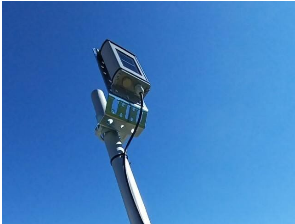
Figure 21: Mounting Plate Parallel to the Pole. Plane of Array (POA) Orientation Shown
