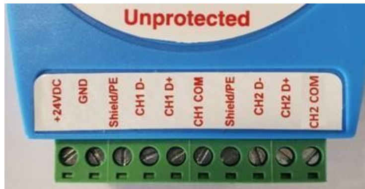
Figure 35: OVP-R2P1 Unprotected Terminals
