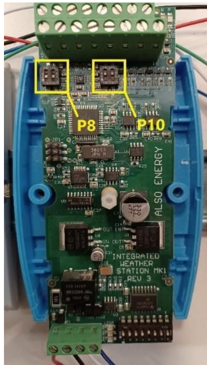
Figure 43: IWS Board Highlighting Gain Switches
