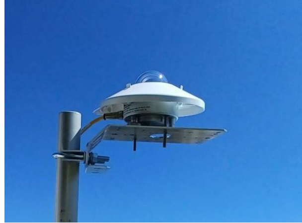
Figure 20: Mounting Plate Perpendicular to the Pole. Global Horizontal Irradiance (GHI) Orientation Shown
