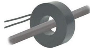
Figure 13: Current Transformer Surrounding Wire
