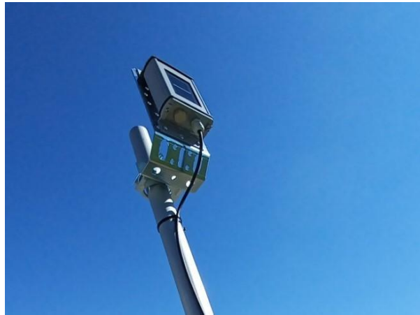
Figure 23: Mounting Plate Parallel to the Pole. Plane of Array (POA) Orientation Shown
