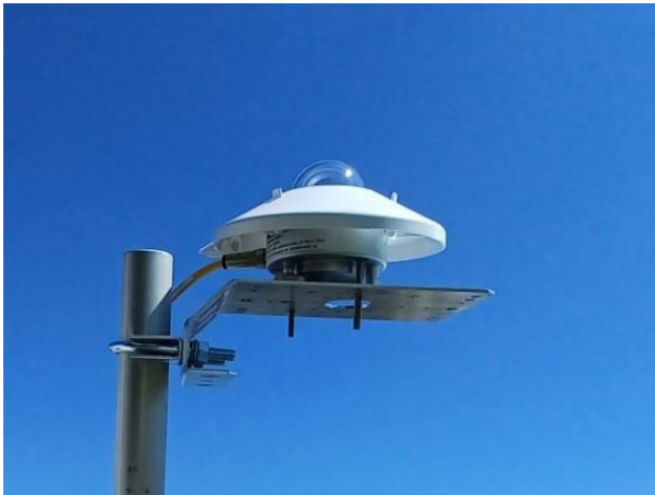
Figure 22: Mounting Plate Perpendicular to the Pole. Global Horizontal Irradiance (GHI) Orientation Shown
